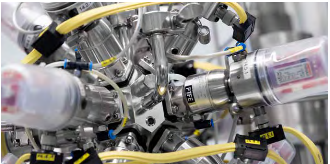
No weld seams (compact design with multi-port body)
