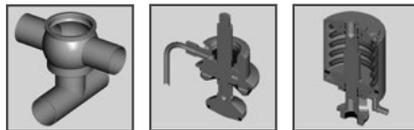
**Asept. Cross Valve** (with Diaphragm [P<sup>3</sup>] and O-Ring - EPDM)
