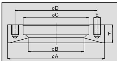
N.b.: Weld-In Flange Z 2000/Select B complies with valve range SVP Model 2000, but is not compatible to the valve range SVP Model 1990!
