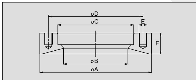
N.b.: Weld-In Flange Z 2000/Select B complies with valve range SVP Model 2000, but is not compatible to the valve range SVP Model 1990!
