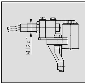
**Mounting Set for Manual Leakage Butterfly Valves**
