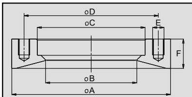
N.b.: Weld-In Flange Z 2000/Select B complies with valve range SVP Model 2000, but is not compatible to the valve range SVP Model 1990!
