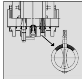
**Control Pin** (including hexagon bolt necessary initial assembly of valve disc 1 with PTFE-laminated seal)
