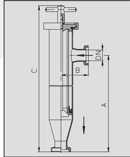
**Angle Type Strainer Combination** (Connections according to DIN 11851)
