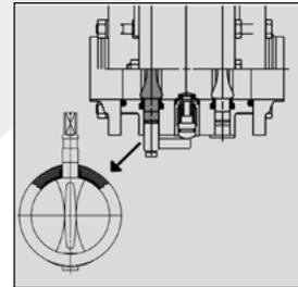
**Pre-Assembled Butterfly Valve Seal (PTFE-laminated EPDM) with Valve-Disc 2**
