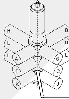
Lower valve housing with clamp connection
