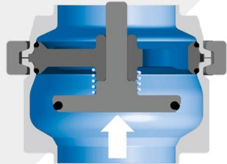
NON-RETURN VALVES P745/P750/P760 / TELLERRÜCKSCHLAGVENTILE P745/P750/P760  $\Delta P [\text{bar}] = \left( \frac{Q [\text{m}^3/\text{h}]}{KV} \right)^2 \Delta P [\text{PSI}] = \left( \frac{Q [\text{gal}/\text{min}]}{CV} \right)^2$
