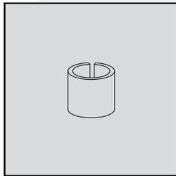
**Bearing Seat for Butterfly Valve Disc** (single piece)\*
